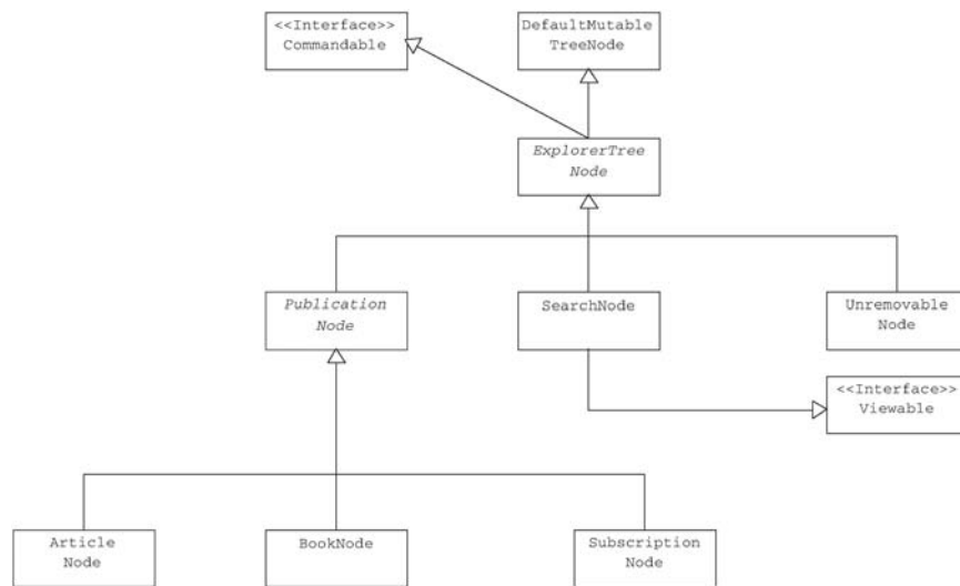
Figure 14.19 Class diagram for the remote explorer's nodes
